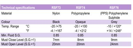
\*Maximum temperature requires ETFE cable to be specified.
