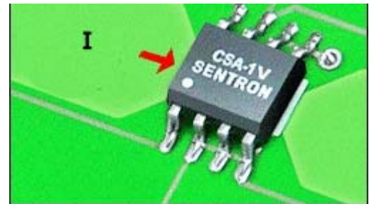
Figure 2 – Sensing current in a PCB trace
